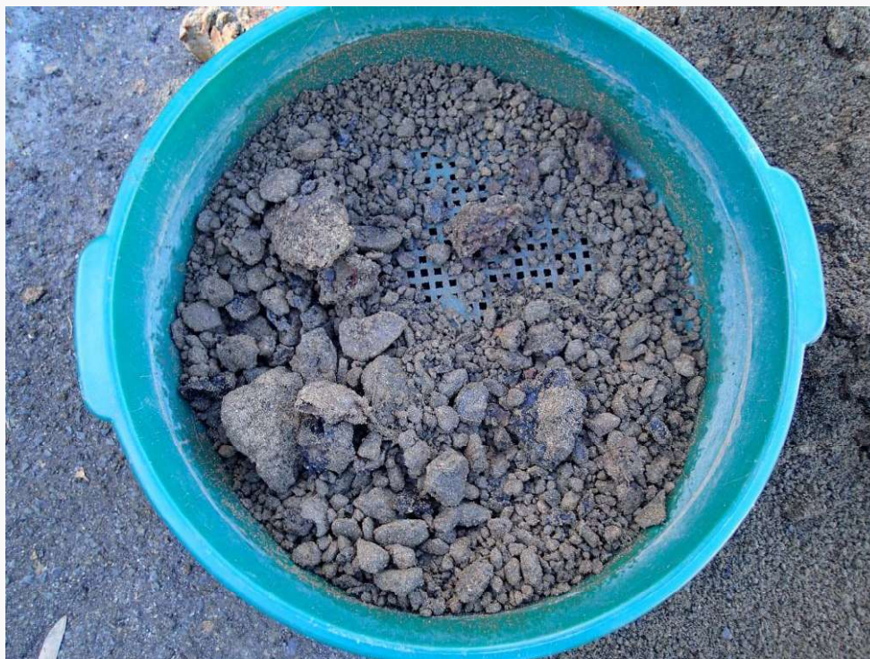
Photo 29: Soil retained on >7 mm sieve from surface sample at location TP13.
