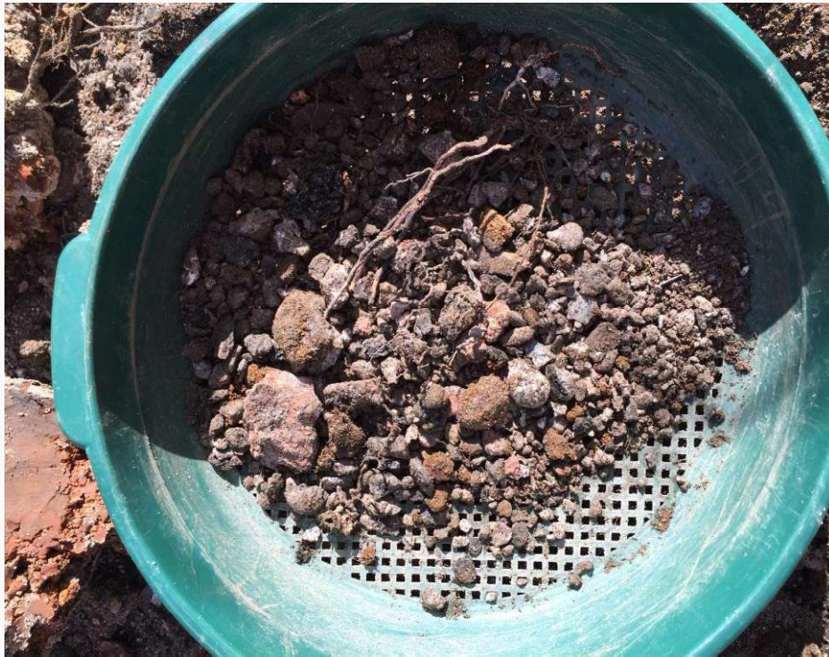
Photo 17: Soil retained on >7 mm sieve from surface sample at location TP01.
